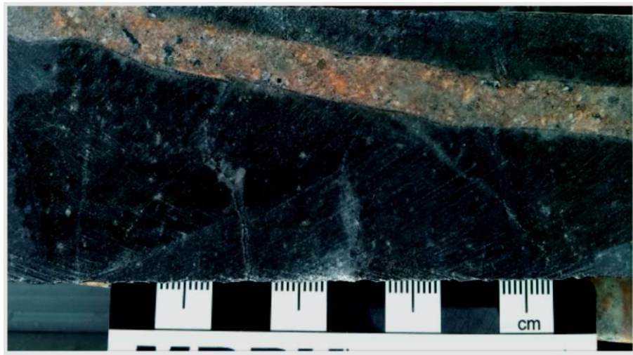
Figure 7.5 Andesitic Tuff, Cut by Quartz-Monzonite-Diorite Porphyritic Micro-Dike. Drill Hole SAC13DDH002, 621.10 m.
