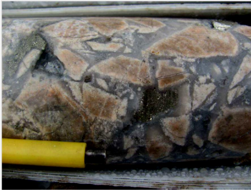
Figure 7.8 Hydrothermal Breccia with Crypto - crystalline Quartz in Drill Hole SAC13DDH001, 351 m Depth.
