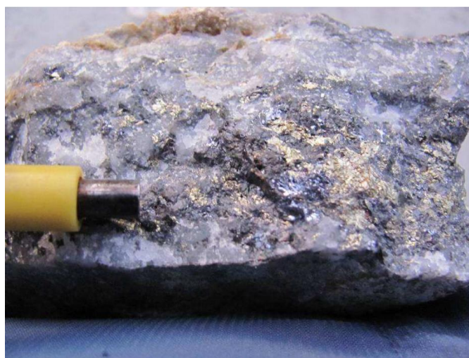
Figure 7.24 Mineralization in El Azul. Milky Quartz – Pyrite – Chalcopyrite – Galena - Sphalerite.
