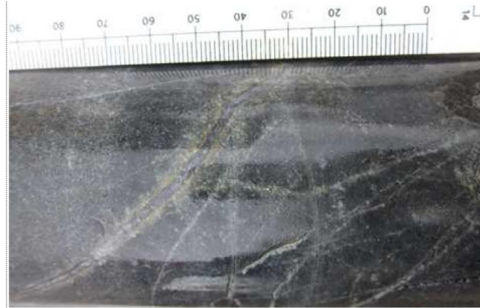
Figure 7.17 Andesitic Tuff with Potassic – Calcic Alteration.
