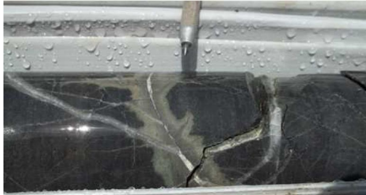
Figure 7.19 Andesitic Tuff with K Feldspar – Sodic Alteration Overprinting the Moderate Secondary Biotite Alteration in Drill Hole SAC13DDH001, 294 m Depth.
